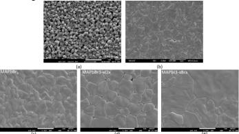
Figure 4. Sample SEM images of (a) solution processed MAPbI3, (b) css processed MAPbI3, (c) css processed MAPbBr3, (d) css processed MAPbBr3-xClx, (e) css processed MAPbI3-xBrx.
