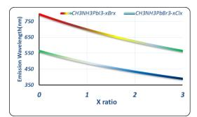
Figure 2. A relationship between the mixture ratio and the emission wavelength.
